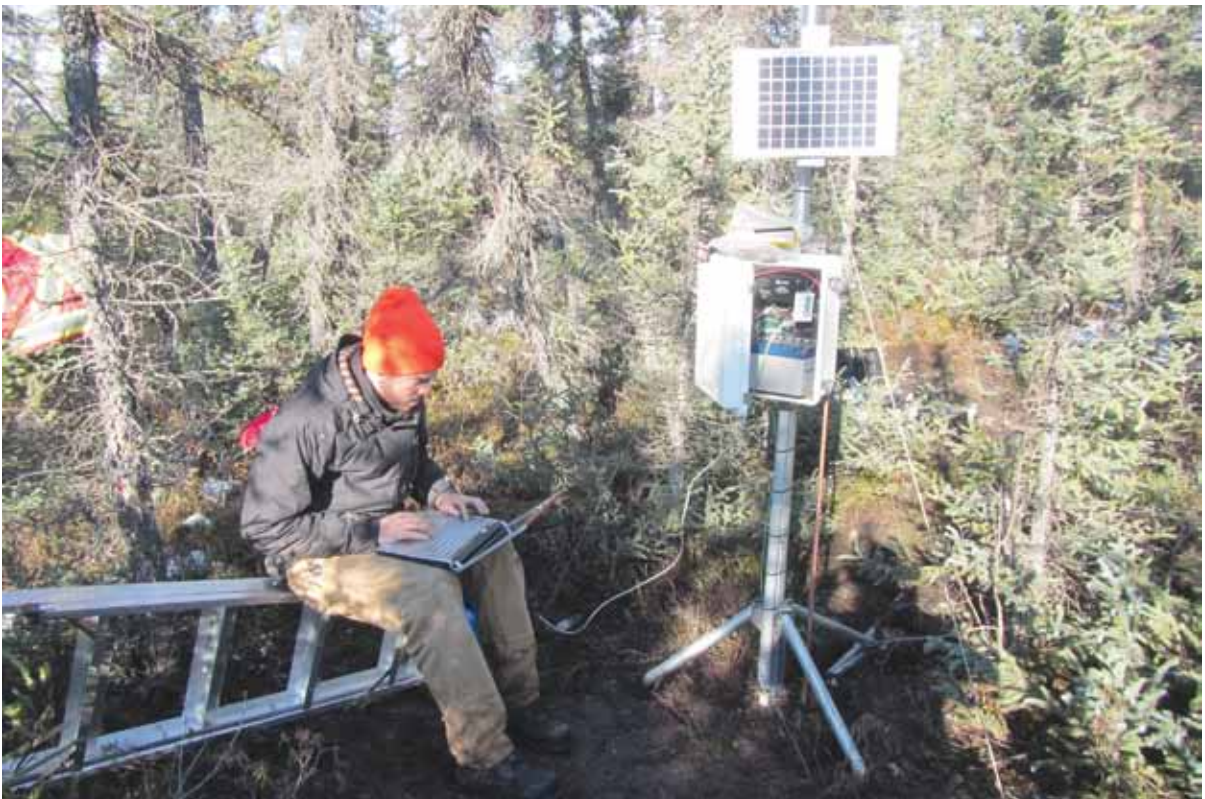
Downloading climate and ground temperature data at BH01, km 1810.2.
