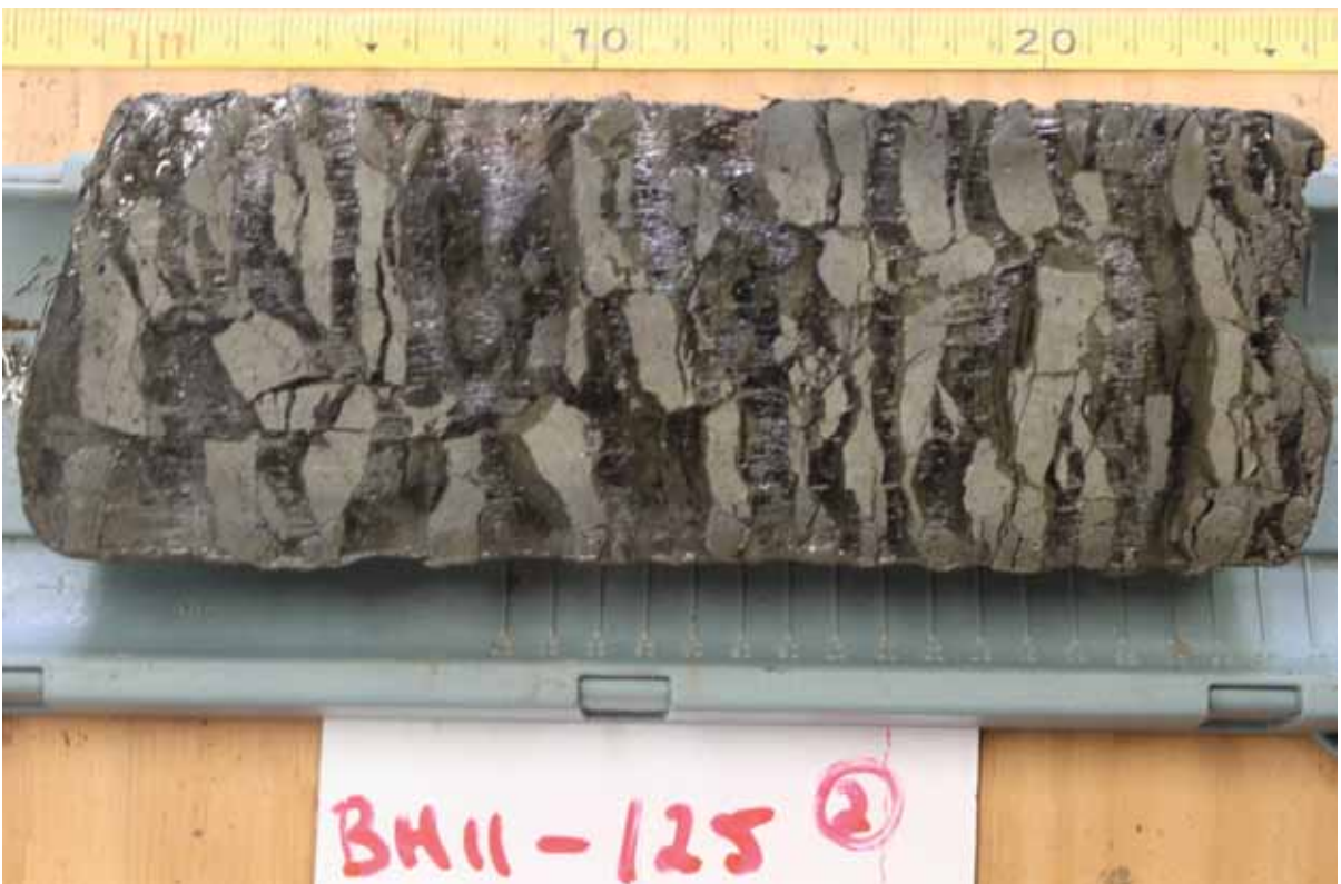
Permafrost core collected at BH11, km 1886.
