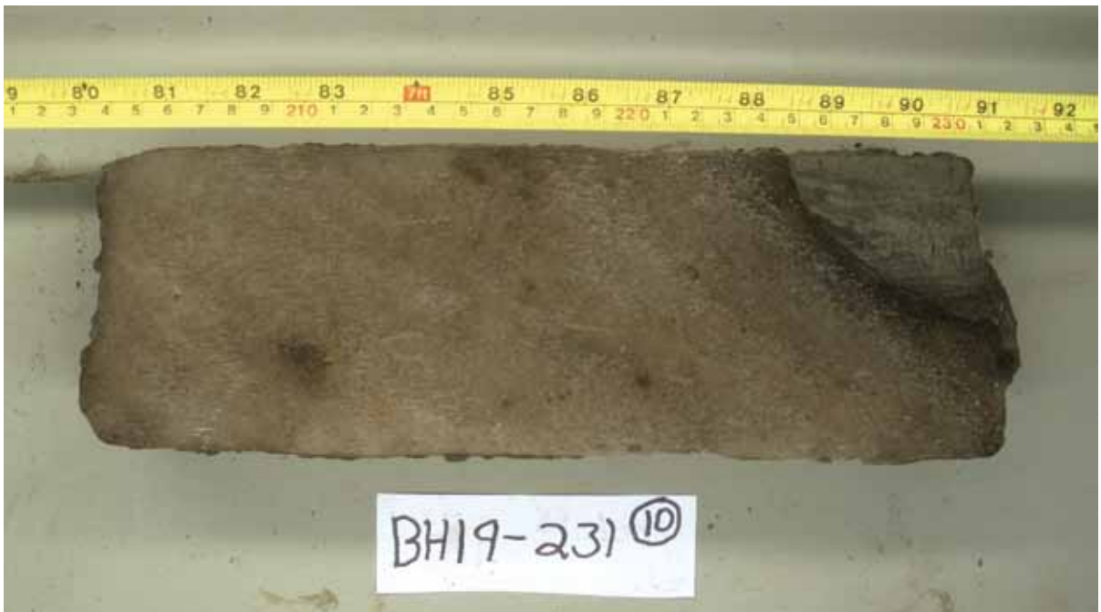
Wedge ice from BH19, km 1862.3.
