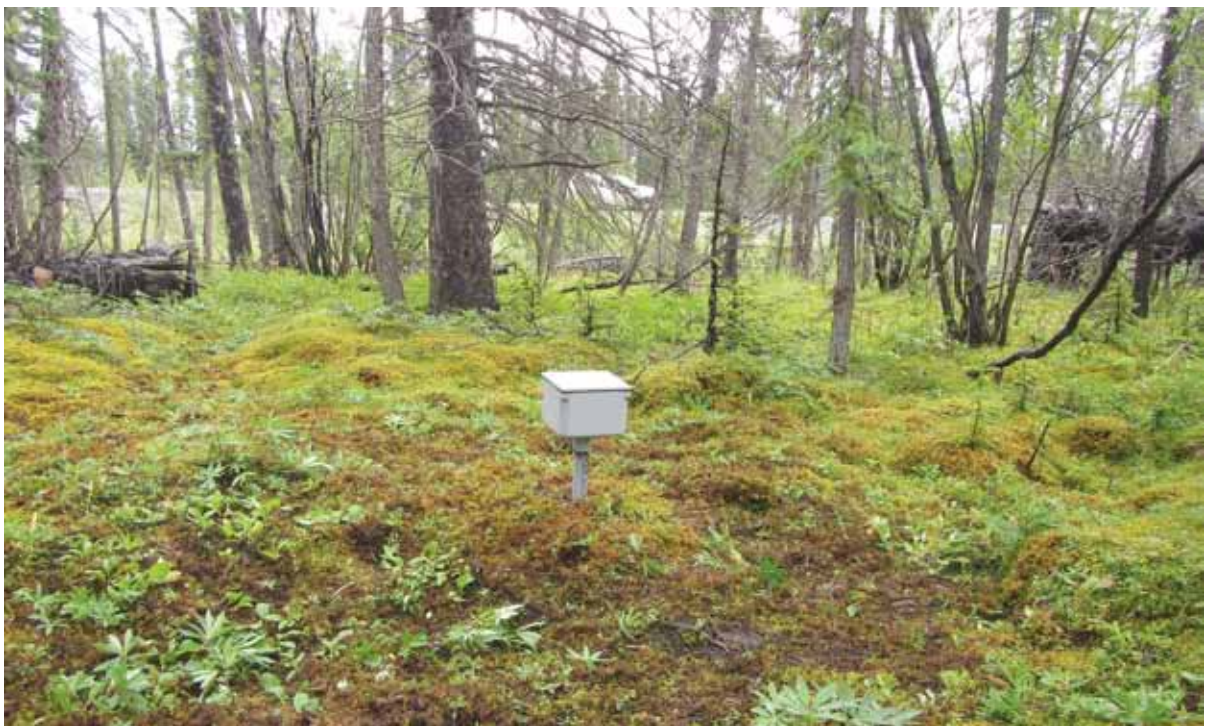
Ground temperature monitoring station at BH08.
