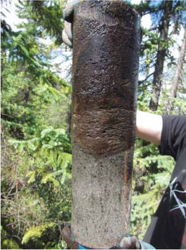
Top of an ice wedge collected at BH13, km 1896.3.
