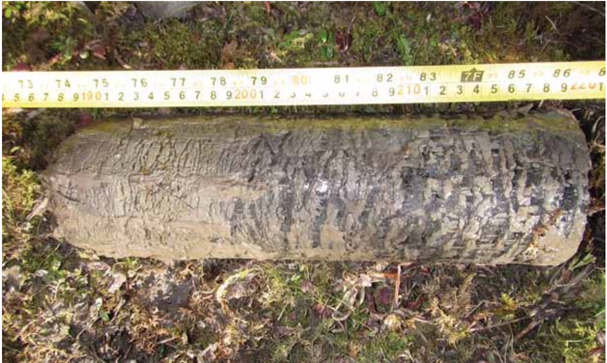
Permafrost core collected at BH08, km 1719.1.
