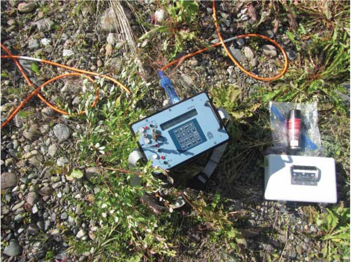
IRIS electrical resistivity system, a one-channel imaging unit.
