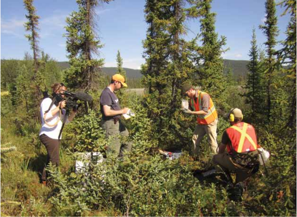
A camera crew films as the research crew extracts and field-logs a permafrost core.
