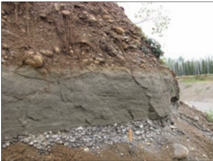
Figure 13. Well-sorted and graded beds of sand-pebble gravel are common deposits in distal glaciofluvial environments.
