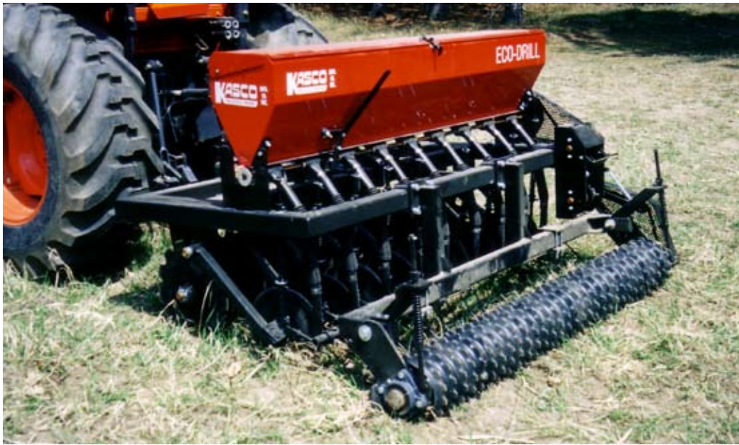
FIG 4.19 This no-till drill seeder has aggressive coulters and a heavy cultipacker and is designed to seed through ground without ploughing. These drills are mainly intended for agricultural and landscaping applications but they are very effective for revegetation sites that have fairly even ground, few rocks and little coarse debris.
