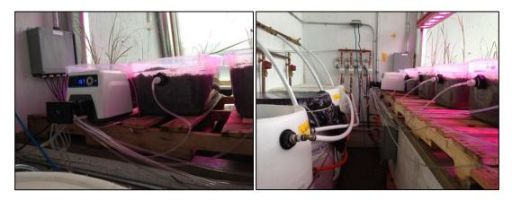
Figure 5 Synthetic influents or tap water being pumped at the bottom of the substrate using a multi-channel peristaltic pump (Masterflex pump, head and C-flex tubing) at 5 ml/min with sub-surface vertical flow.
