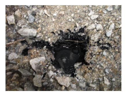
Figure 9 Black deposits on the wetland surface, characteristic of sulfide precipitates found only in the Pit(MeOH) CW treatment. In addition, an odiferous evidence of  $H_2S$  from the Pit(MeOH) was present.
