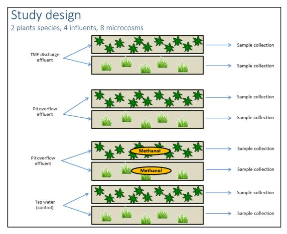
Figure 1 Constructed Wetland (CW) study design using two plant species (*Carex aquatailis* and *Juncus balticus*) and 4 different synthetic influents (TMF, Pit, Pit(MeOH) and Control) for a total of 8 laboratory-scale CWs.
