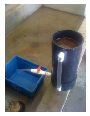
Figure 4 Hydraulic conductivity testing to determine the appropriate ratio of peat, sand and pea gravel to achieve a 5 ml/min flow rate with a hydraulic residence time of approximately 5 days.
