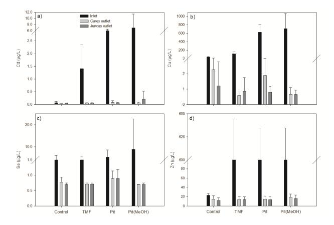
Figure 6 Cd (a), Cu (b), Se (c) and Zn (d) concentrations in CWs with C. aquatilis (Carex) and *J. balticus* (Juncus) fed with Control, TMF, Pit or Pit(MeOH) waters. Bars represent means with standard error. There were no significant differences in the outlet concentrations for any of the contaminants between the wetland treatments (repeated measures ANOVA with Tukey posthoc (p>0.05 for all comparisons). Note the broken Y-axis.
