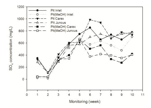
Figure 8 Sulfate concentration in the inlet and outlet waters of the Pit and Pit(MeOH) CWs with *C. aquatilis* (Carex) and *J. Balticus* (Juncus) monitored over the 10 week trial. Significantly higher sulfate consumption (i.e. Inlet-Outlet for each CW) for both Pit(MeOH) CWs compared with the Carex Pit treatment were detected (ANOVA with Tukey posthoc, p=0.05 for Carex and p=0.02 for Juncus).
