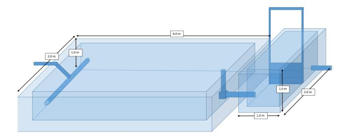
Figure 4: Proposed cell and weir channel construction with measurements
