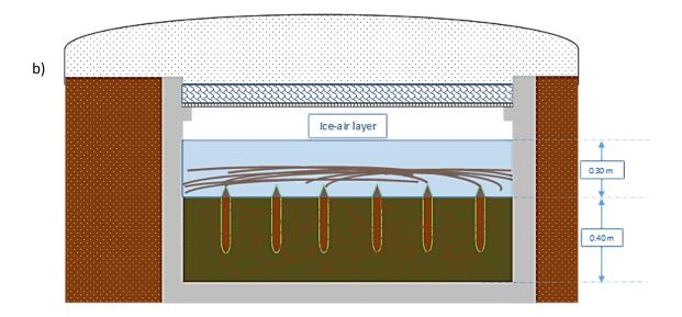
**Figure 7**: Implementation of ice-air layer to increase insulation of wetland cells. Note a) demonstrates flooding of the cell and placement of reinforcing metal mesh just prior to sub-zero temperatures and b) demonstrates the formation of a reinforced metal-ice layer following a decrease in cell water level.
