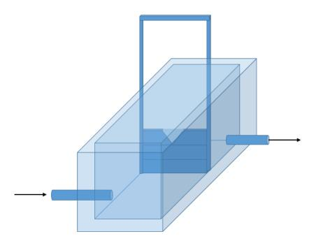
**Figure 6**: Proposed design for V-notched weir to control water level in preceding cell and determining flow rate.
