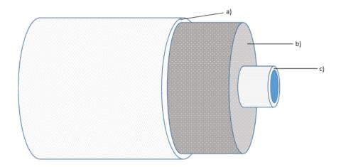
**Figure 5 -** Illustration of potential pipe insulation to guard against cold and precipitation. Note a) outer PVC pipe, b) pipe insulation, and c) inner PVC pipe accommodating the flow of water.
