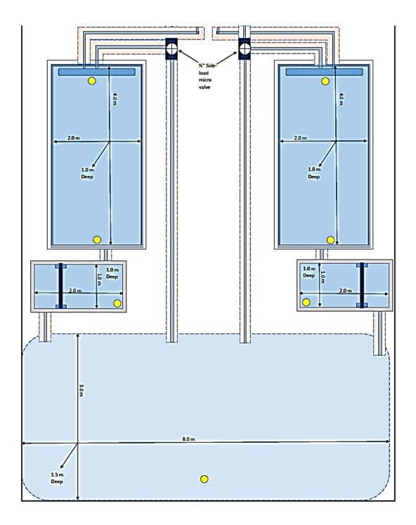
**Figure 3**: Design for northern passive treatment research facility with sizes. Yellow circles indicate potential placement areas for multi parameter sondes.
