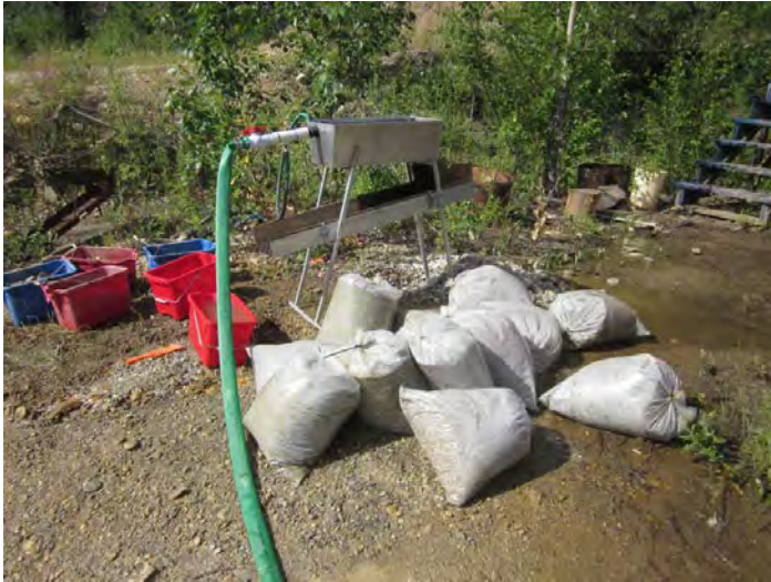
Figure 43 - Bags of Sluicibox Tailings Collected by Hand which are ready for processing on the author's very well tested testing sluice.
