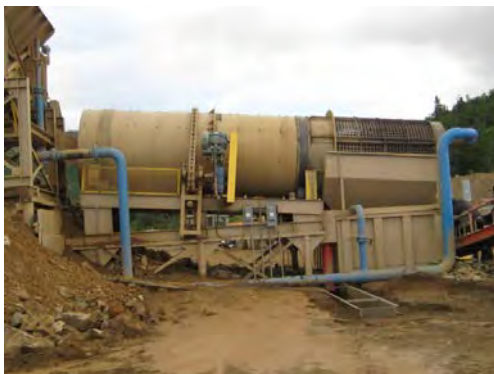
Figure 68 - High Speed Rubber Lined Trommel to Scrub Clay-Rich Gravels.
