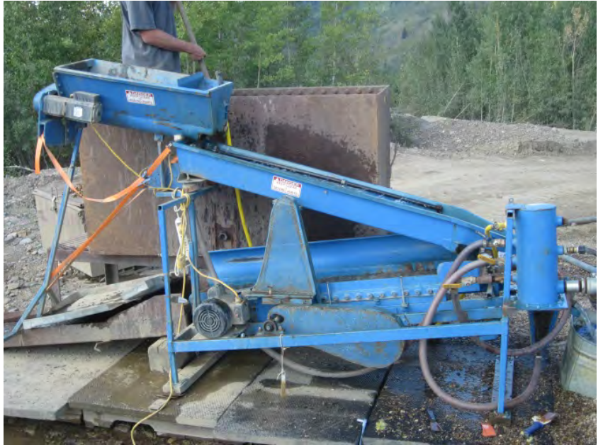
Figure 25 -Top View of Lizotte Live Bottom Sluice with Feeder, Vibrating Screen Deck and Live Riffles.
