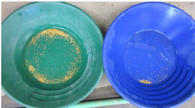
Figure 48 - Test Sluice Concentrates were hand panned to raw gold where possible or to a final concentrate for later lab testing. Gold samples were cleaned dried and weighed.
