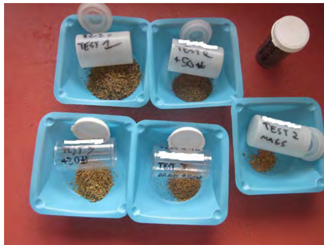
Figure 81 - Cleaned gold from mines with abundant galena in their concentrates.
