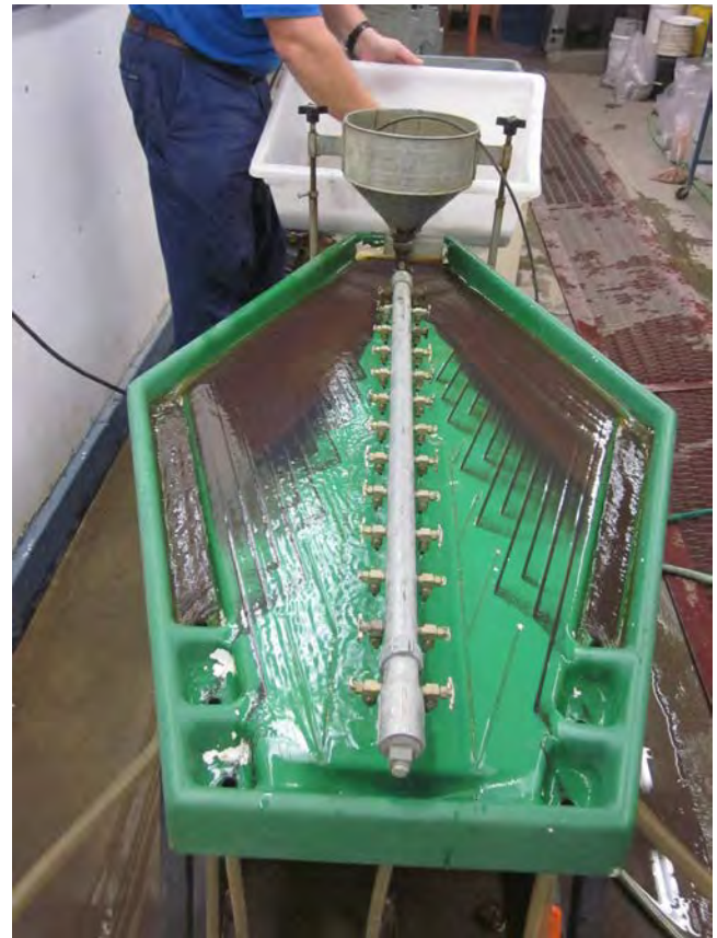
Figure 33 - Keene ST1 Shaking Table with Rotating Magnetic Separators with Simple Feeder Mounted on Steel Base with Sand Bags.
