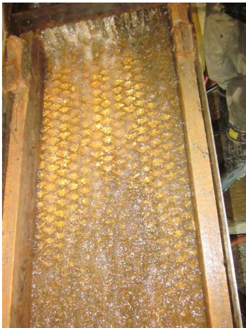
Figure 24 - Long Tom with Gold at Top. Riffles.
