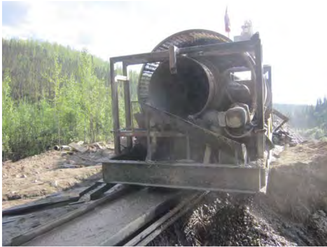
Figure 62 - Above – Surging in Sluice Run at the End of the Reverse Spiral Trommel.
