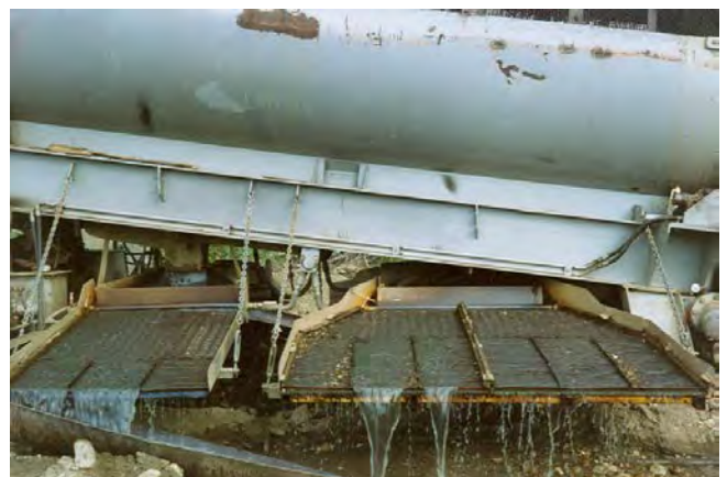
Figure 73 - Sluice Runs Too Short With & No Angle Iron or Hydraulic Riffles
