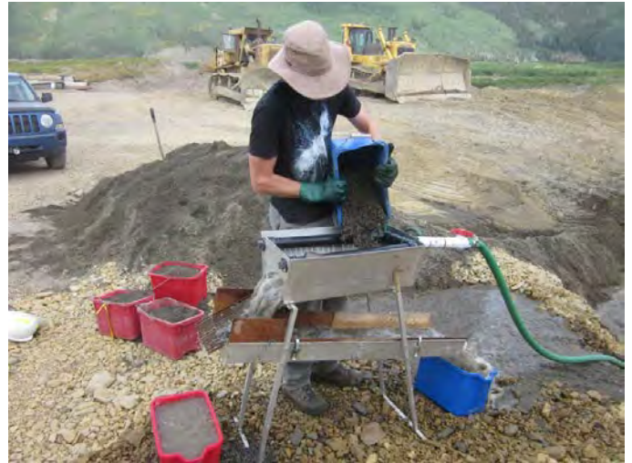
Figure 47 - Gavin Clarkson Processing Sluicibox Tailings Sample on Author's Testing Sluice.
