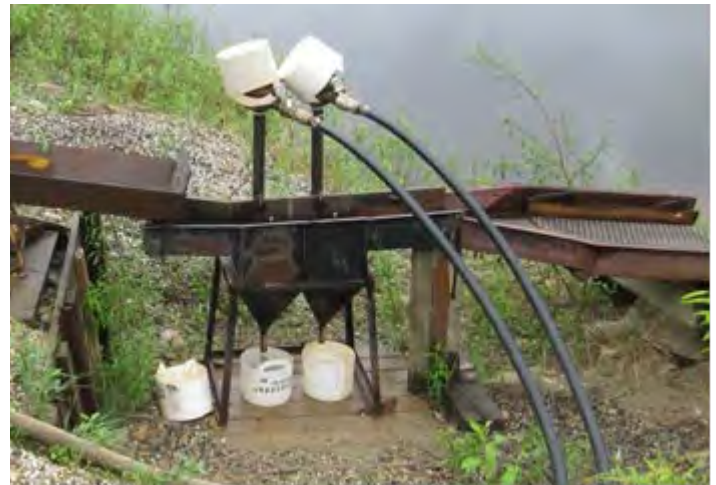
Figure 27 - Typical Dual Cell Hydraulic Operated Jig with long tom at the discharge to recover fine gold typically lost by this type of jigging system.
