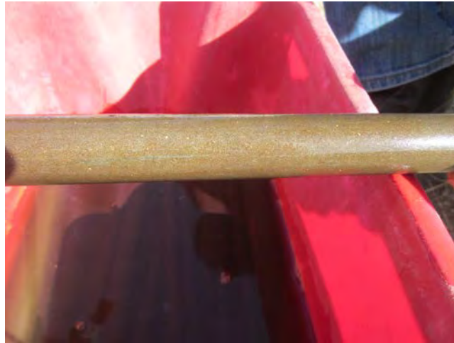
Figure 89 - Rod with pits in filled with gold.
