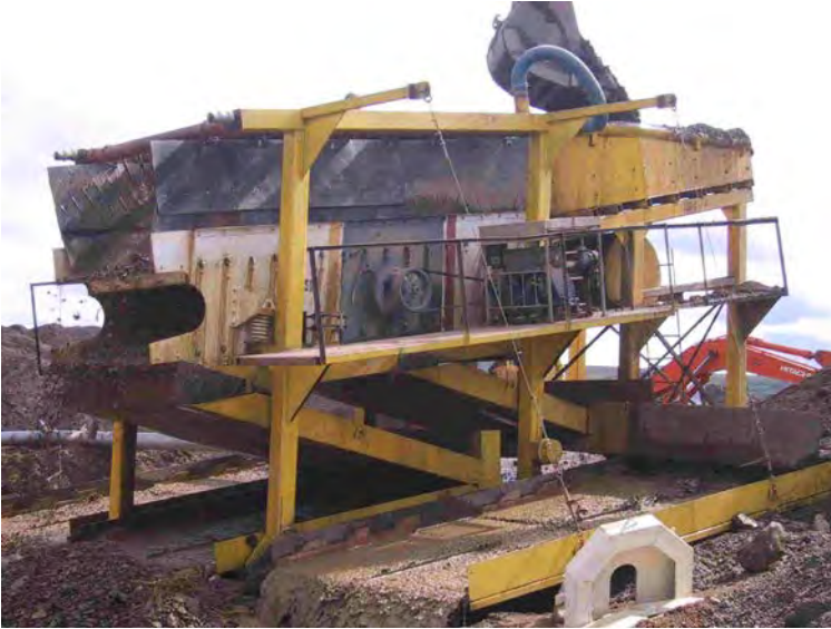
Figure 20 - Pre-Screened "Z" Box.
