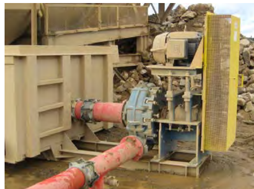
Figure 69 - Rubber Lined Gravel Pump Breaks Down Clay.
