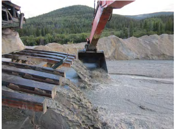
Figure 44 - Collecting Live Sluicibox Tailings samples with an Excavator.
