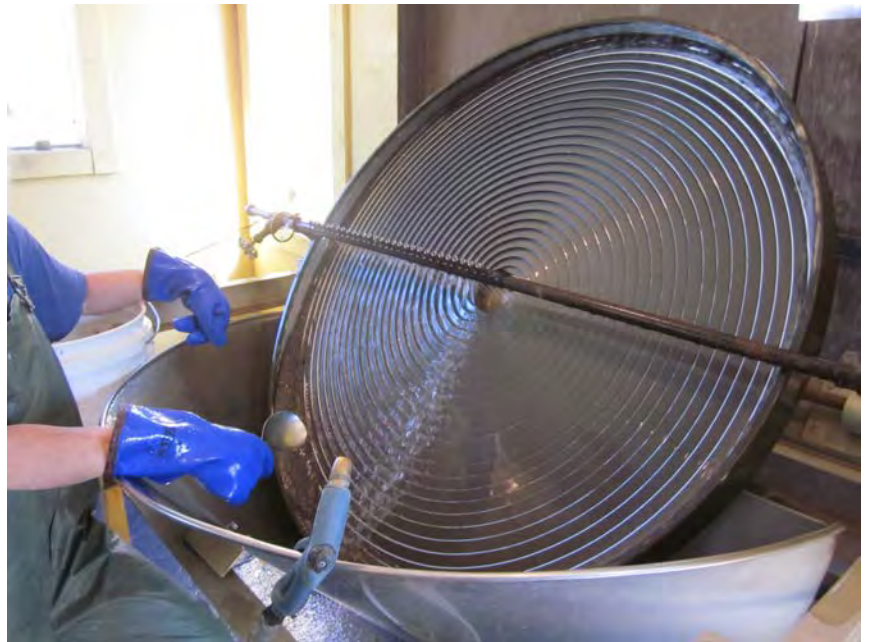
Figure 29 - Large Diameter Gold Wheel - Bulkier gold particles travel up the Spiral to the Center and discharge out behind the center of the wheel.
