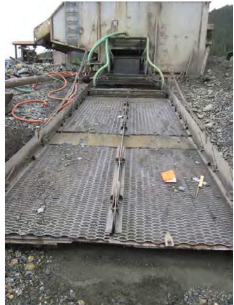
Figure 70 - Above - Good Design with Hydraulic Riffles at Top and Slick Plates between Sections of Coarse Expanded Metal Riffles.
