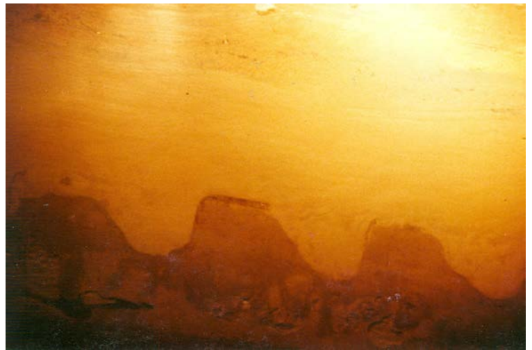
Figures 18 & 19 - Cross-section schematic and photo of one inch angle iron riffles in operation. Note: Due to their higher density, gold particles tend to segregate to the bottom of the slurry flow where they form a streamline that is diverted by a low-pressure zone into a riffle to form a vortex. At the bottom of this vortex gold particles are driven into the matting.
