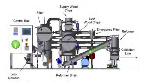
The reactor supports changing the wood chip fuel into wood gas. At the pyrolysis zone, the wood decomposes and begins reducing from its visible wood state. The fuel is then converted to a coal-like hydrocarbon and transported to the oxidation zone where part of the carbon is burned with injected air at approximately 800°C. As the gases move over the hot ember bed (oxidation zone) the tar and hydrocarbons are separated from the gas, resulting in a gas with very low tar.
