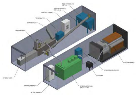
Figure 4.1 Potential Proton Power Containerized 500 kW<sub>e</sub> Units
