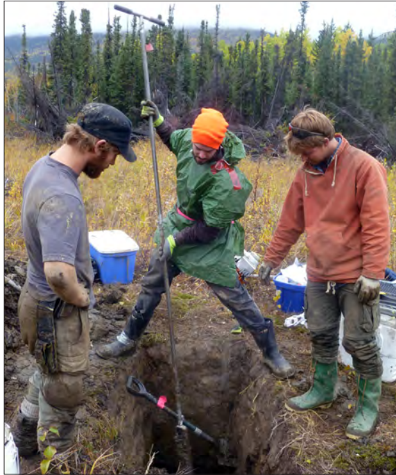
Figure A2. Photograph of the hand auger, used for permafrost coring.
