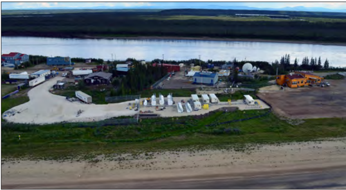
Figure 33. Thick aggregate building pads are an example of anthropogenic deposits in Old Crow. The airport is the biggest continuous area composed of anthropogenic materials, and much of the downtown core contains anthropogenic deposits of aggregate.
