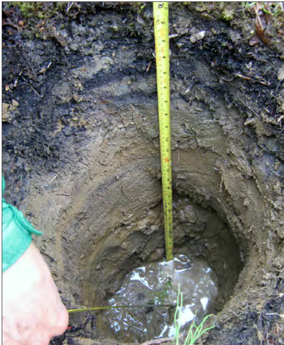
Figure 20. This soil pit dug in the back-channel part of the floodplain in Old Crow (near the ski trails) has fine, silt-rich soil and a shallow active layer. At this site, the water table was encountered 45 cm below the top of the moss mat where it was perched above a ~65 cm deep permafrost table.
