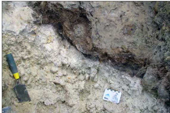
Figure 24. Organic material (dark brown) and altered parent materials (white quartz sand) at the top of the high-level gravel where it is buried by ~5 m of diamict.
