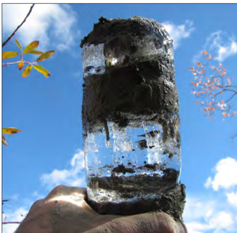
Figure C6. Example of ice-rich permafrost core from the Beaver Creek area, Yukon.
