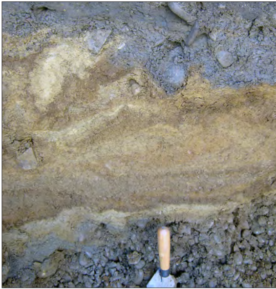
Figure 27 (left). Silt-rich diamict is the highest stratigraphic unit on the escarpment above town and is interpreted as a colluvial deposit generated on the pediment slope above. The thickness of this unit is thought to be controlled by the depth of cryoturbation that occurs in the active layer above the permafrost table. The underlying sand unit in this photo has disturbed bedding near its contact with overlying silt, but relatively undisturbed beds below where they have been preserved by permafrost.
