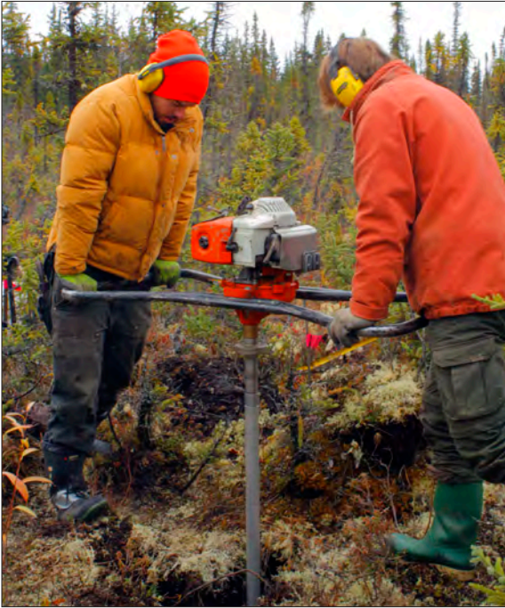
Figure A1. Photograph of the GÖLZTM portable core-drill system used for permafrost coring.
