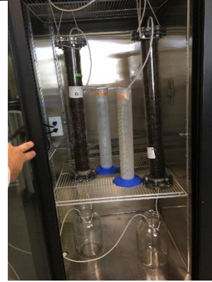
Figure 1. (a) Schematic of column design and experimental setup. (1) influent (SMW); (2) peristaltic pump; (3) column; (4) effluent. Schematic is not to scale. (b) Picture of actual experimental setup located in the Yukon U Research Centre Laboratory.
