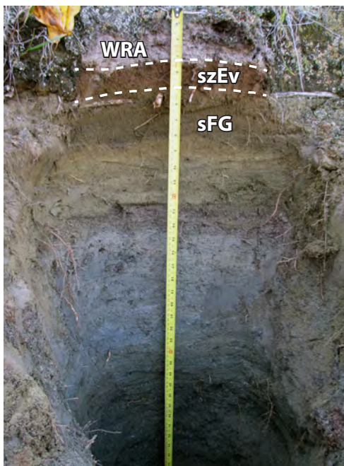
Figure 39. Soil pit located at the top of the escarpment behind the radio tower, approximately 200 m west of Del Van Gorder School (station 14PL049). Over 1 m of glaciofluvial sand ( sFG ) underlies 7 cm of White River ash ( WRA ) and 5 cm of red-brown loess ( szEv ).
