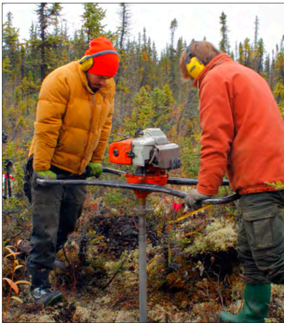
Figure A1. Photograph of the GÖLZ™ portable Earth-drill system used for permafrost coring.
