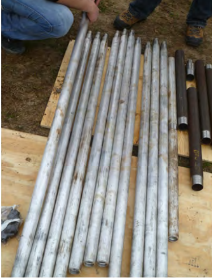
Figure A3. Photograph of aluminum rods used for the Winkie drill for permafrost coring.
