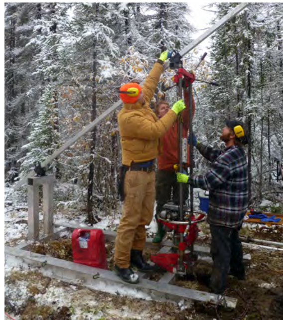
Figure A2. Photograph of the Winkie drill, used for permafrost coring.
