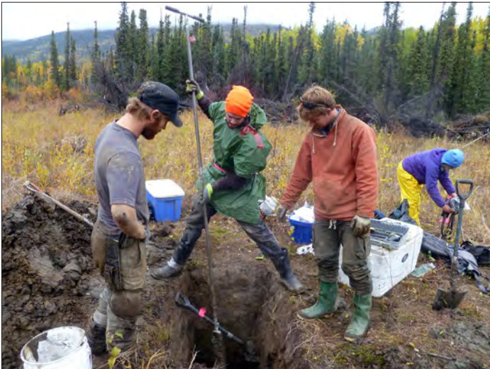
Figure A5. Photograph of the hand auger, used for permafrost coring.
