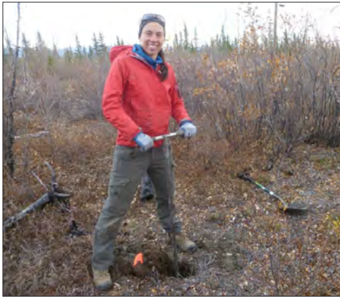
Figure F5. Frost-probing to determine depth to permafrost.
