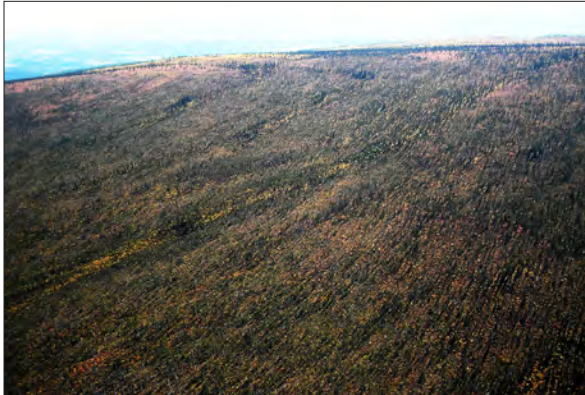
Figure 20. Typical surface expression indicating the presence of sheetwash on a north-facing slope underlain by permafrost.
