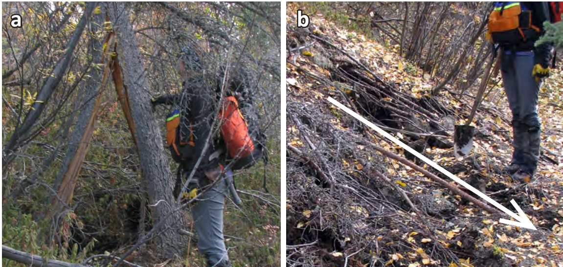
Figure 47. (a) Split tree (station WPT714 on Fig. 19a) and (b) fresh tension cracks emphasized by pulled roots (station WPT715 on Fig. 19a) indicate active instability on the southwest-facing slope immediately south of the ski hill.
