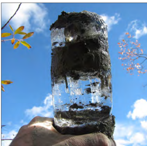
Figure F6. Example of ice-rich permafrost core from the Beaver Creek area, Yukon.
