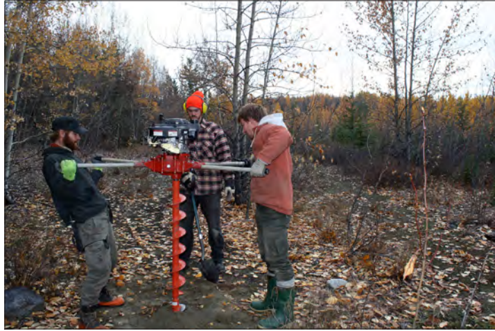
Figure A4. Photograph of the Honda drill, used for permafrost coring.
