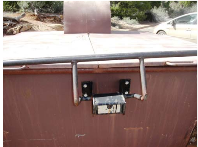
Figure 11: This locking bar mechanism, manufactured by Serious Industries, has been bolted on a conventional dumpster and shown here at Mesa Verde National Park, to deter black bears. Photo credit: S. Gilbert
