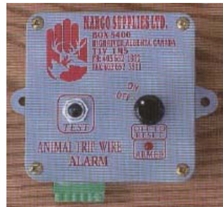
Figure 12: Example of a trip wire alarm controller supplied by Margo Supplies Ltd. Photo credit: Sowka 2013, p. 6-3.
